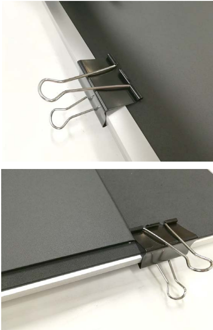
Figure 9: Different possibilities to use double paper clamp to hold the substrate
